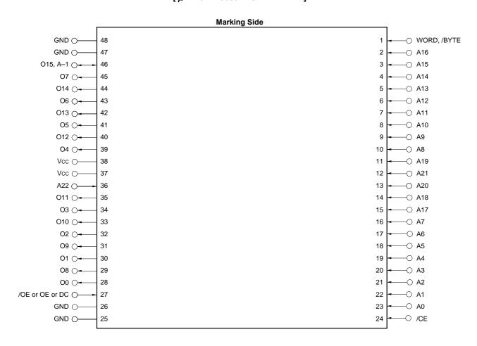
A0 to A22 : Address inputs O0 to O7, O8 to O14 : Data outputs
