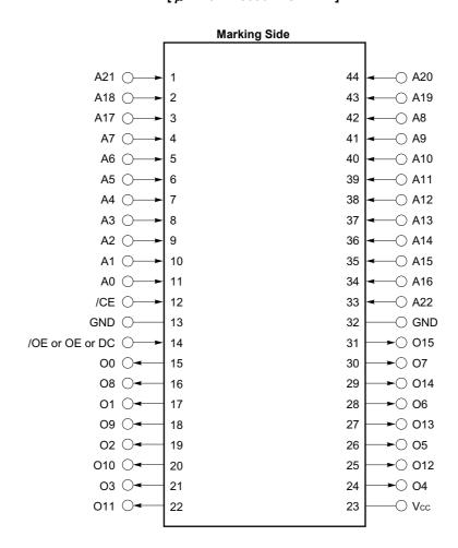
A0 to A22 : Address inputs O0 to O15 Data outputs /CE Chip Enable /OE or OE Output Enable Vcc Supply voltage **GND** Ground DC
