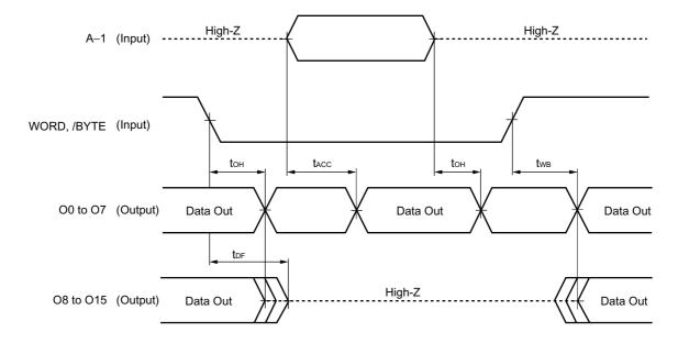
Remark Chip Enable (/CE) and Output Enable (/OE or OE) : Active.
